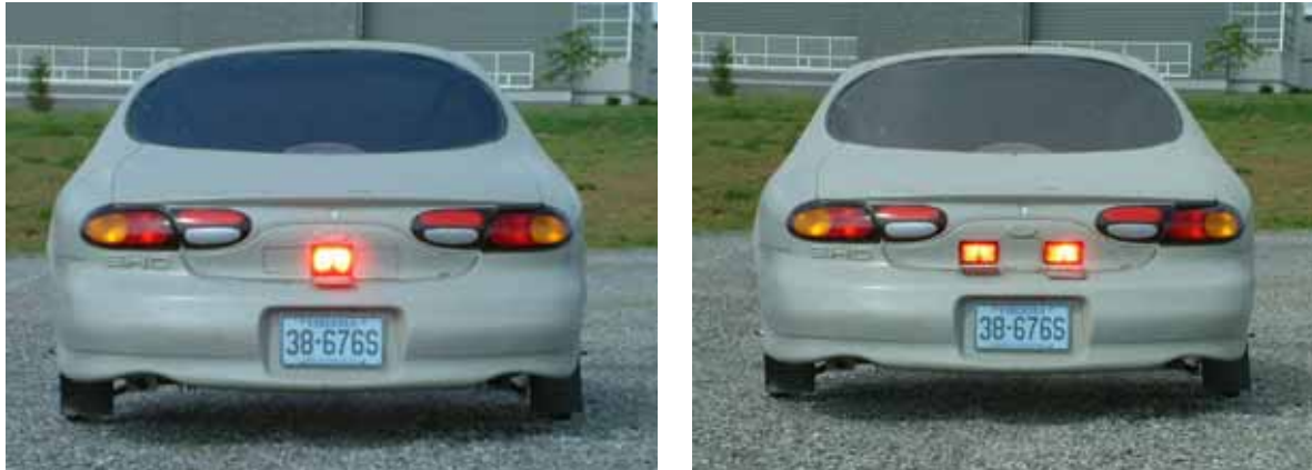
Figure ES1. The TCL (left) and IAP (right) imminent-warning lighting signals as used in the Task 3 Experiment of the previous study.
